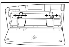
**2** Adjust the paper width guides to the width of the envelope.
